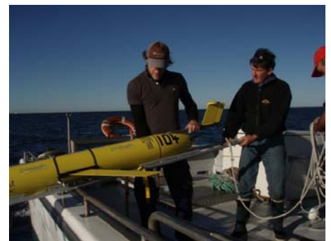
Ocean gliders dropped into the ocean on the North West shelf
